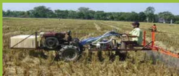
Power Tiller Mounted Sprayer
