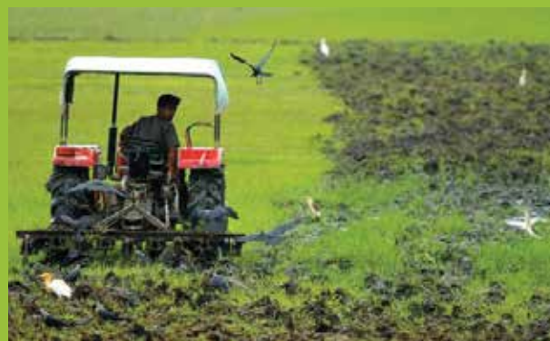
Field Operation of Tractor Drawn Disc Plough
