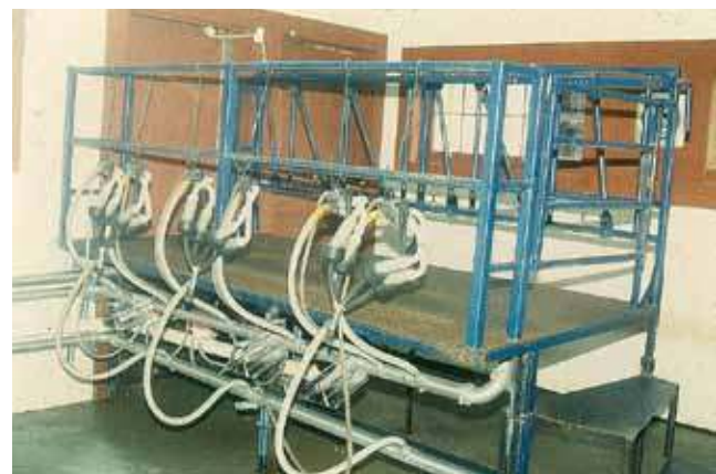
Photo 9.6 Prefabricated elevated parlor.
