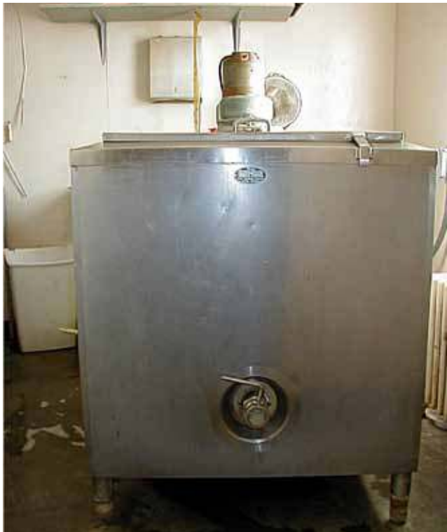
Photo 11.2 100-gallon ice bank bulk tank.
